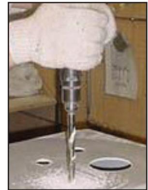
Using a drill with a positive rake angle and thin points or split points can help reduce cutting pressure and thus delamination at both entrance and exit. Feed rates must also be constant and may even be reduced upon exiting from a hole to reduce flexing of the part when the drill exits. Using a solid back surface to support the part when drilling can also aid in reducing delamination and chipping.
